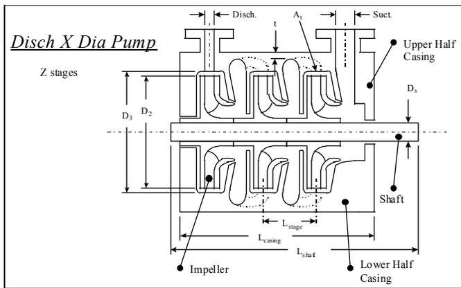
Figure 1. Simplified Centrifugal Pump Embodiment
